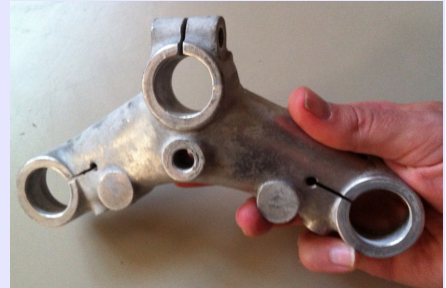
The original triple. A crack near the top bolt mean this part was no longer serviceable.
