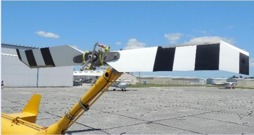
Our client has been fabricating composite blades for helicopters tail rotors for decades, using very unique tooling that was constructed in the early days of CNC. That means that the original digital data that was used to cut the unique shape of the molds was lost long ago, so building new molds to support their growing demand means they first need to create new 3D models of their existing rotors.
