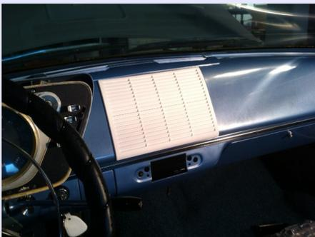
We chose to use a sintered nylon 3D printing process to capture the fine detail of the original grill, while providing a strong, flexible part that could be installed in the vehicle without breaking. The new part snapped perfectly into place, and hugged the contours of the dashboard as it was originally designed. With a little hand sanding, the new grill would soon be ready for paint and final finish. A beautiful application of 3D scanning and 3D printing, bringing a new life to aging plastic.
