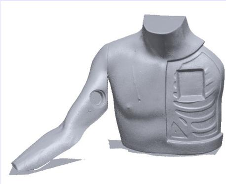
The form came to our shop in two pieces. The torso and arm were separate, but joined together with a single bolted fastener. We first scanned each piece separately in order to capture all of the mating surfaces, and then performed a second scan as an assembly, to ensure that both pieces would be aligned correctly in the new digital reconstruction.
