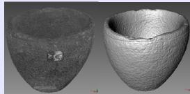
We chose not to use any surface treatment for the demonstrations scans. Materials like stone scan exceptionally well with structured light technology, and there was no need to prepare the surface. We used the HDI Advance R2, configured to capture 12" and our automated rotaery table to complete the scan quickly, and with stunning detail.
