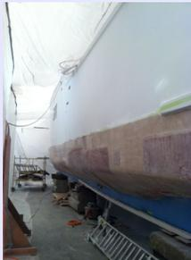
Big boats are challenging enough, but a big boat in a small space introduced some new challenges. We first removed most of the build up and scaffolding around each boat so that there was a clear line of site for the scanner. We then took a series of 3D scans from various positions around the boat, from the ground and from a 30' man lift available on site.
