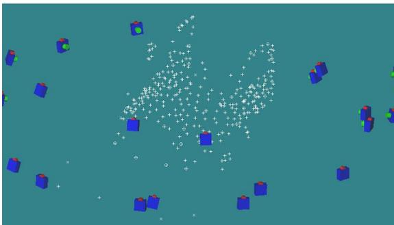
Once the photo images were digitally processed and aligned, we could then generate a reliable skeleton of all of the markers positioned in 3D space. The software first calculates the position of the camera for each image, and then uses the
